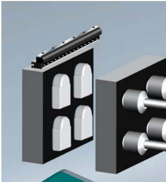
High speed ionised air is blown down toolface as soon as it opens to kill the charge and release the mouldings
