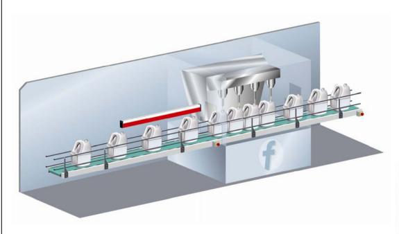
If misbehaviour of the container is also an issue then 1250-S Bars can be positioned either side of the conveyer to prevent problems from occurring before the filling stage.
