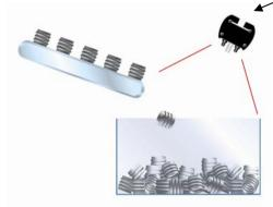
A 3850 Ionstorm Bar (or 2000 / 2020 Ionised Air Blowers) will neutralise the charge in the closures to prevent dust attraction, shocks to operators and product misbehaviour.
