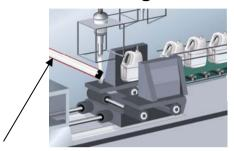
A 3850 lonstorm Bar positioned at a distance of up to 500mm neutralises the parison and prevents it being attracted to the tool. It generates no air movement and because of its long distance performance can be positioned away from the moving machinery.
