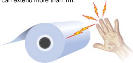
The electric field around reel can extend more than 1m.
