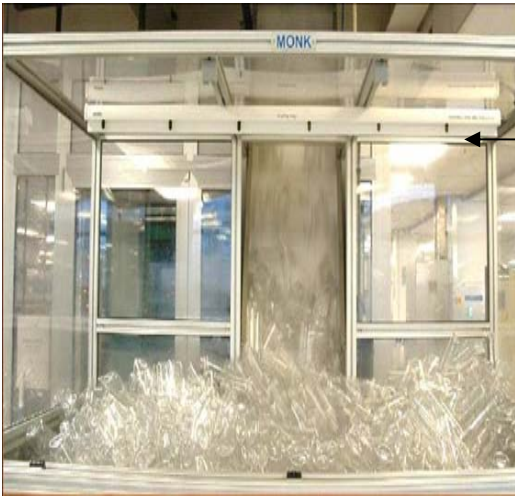
A large hopper of plastic bottles was giving shocks to operators at a distance of up to 1m.
